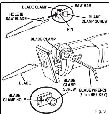
**Note:** There may be times when the blade clamp sticks to the saw bar and will not loosen enough to allow blades to be installed or removed. If this happens, loosen the blade clamp screw with the blade wrench, then tap lightly on the end of the blade wrench with a mallet. See Figure 4.
