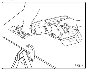
Mark the line of cut clearly. Choose a convenient starting point inside the area to be cut out and place the tip of the blade over that point. Rest front edge of base (shoe) assembly on work and hold firmly in position. Depress the lock-off button, then pull switch trigger to start the cutting action.
