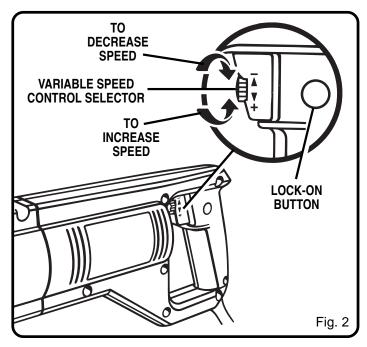
the switch trigger, push in and hold the "lock-on" button, then while holding the "lock-on" button pushed in release the switch trigger. Next, adjust the variable speed control selector until the desired speed is reached.
