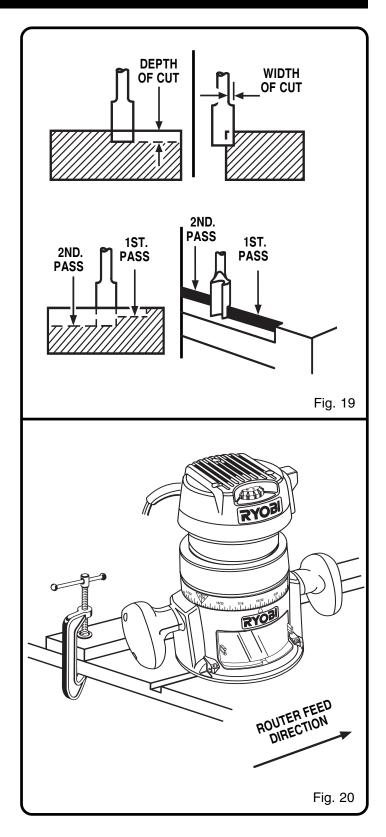
When routing a groove wider than the diameter of the cutter, clamp a straightedge on both sides of the cutlines. Position both guides parallel to the desired line of cut and spaced equal distances from the desired edges of the groove. Rout along one guide; then, reverse direction and rout along the other guide. Clean out any remaining waste in the center of the groove freehand.
