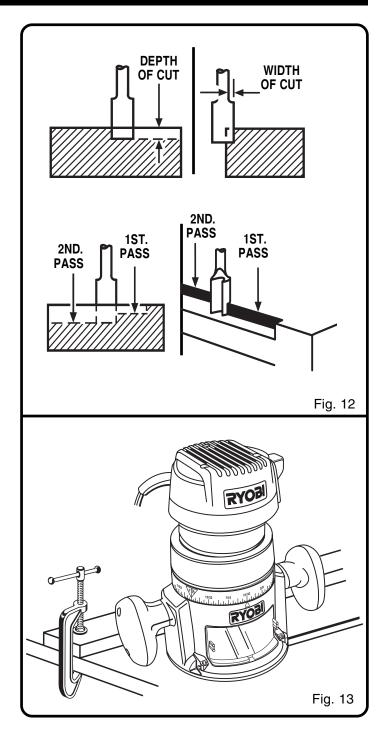
When routing a groove wider than the diameter of the cutter, clamp a straightedge on both sides of the cutlines. Position both guides parallel to the desired line of cut and spaced equal distances from the desired edges of the groove. Rout along one guide; then, reverse direction and rout along the other guide. Clean out any remaining waste in the center of the groove freehand.
