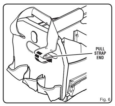
Secure pull strap by fastening end to snaps located on inside of toolbox.
