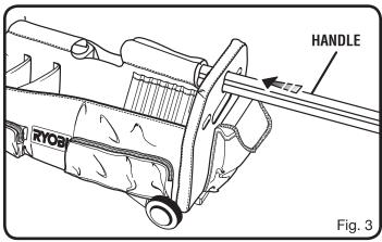
Thread handle through the sleeves in the center divider section and seat in the vertical opening on the opposite side of the frame.
