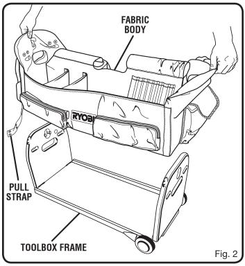
Insert the toolbox handle through the vertical opening located on the end panel of the toolbox frame.
