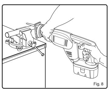
**Never** use gasoline since normal sparking of motor could ignite fumes. Clamp the work firmly and cut close to the clamping point to eliminate any vibration of the work being cut. When cutting conduit pipe or angle iron, clamp work in a vise if possible and cut close to the vise. To cut thin sheet material, sandwich the material between hardboard or plywood and clamp the layers to eliminate vibration and material tearing.
