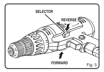
This tool has the feature of being reversible. The direction of rotation is controlled by a selector located above the switch trigger. With the drill held in normal operating position, the direction of rotation selector should be positioned to the left of the switch for drilling. The drilling direction is reversed when the selector is to the right of the switch.
