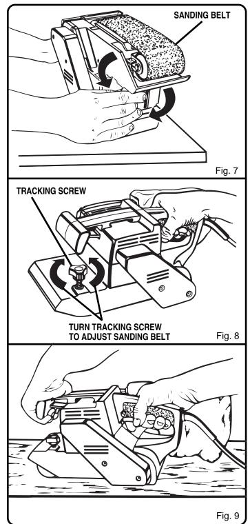
Your sander was designed to provide the proper weight on the sanding belt. Extra pressure will result in uneven work, clogged belts, and possible motor burnout. **NOTE:** The front roller of your sander was not designed for contour sanding. Sanding on the front roller could cause irregularity in sanding belt tracking.
